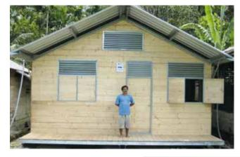
Painted house in Nias, Indonesia. Due to the difficult terrain in which to construct, the situation in Nias required a different type of housing from that used in Aceh. Instead of a reinforced concrete construction, the Canadian Red Cross used an expanded transitional shelter approach (33m2) that allowed for stable construction on uneven ground, easy portability and maintenance of quality control. Each house took two to three days to build.
